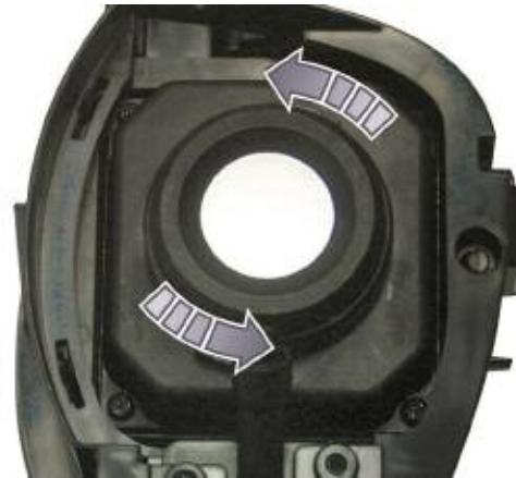
Replacing front lens
